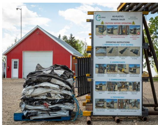
Silage plastic, densified & prepared for transport using the manual compacting system. Source: Cleanfarms
